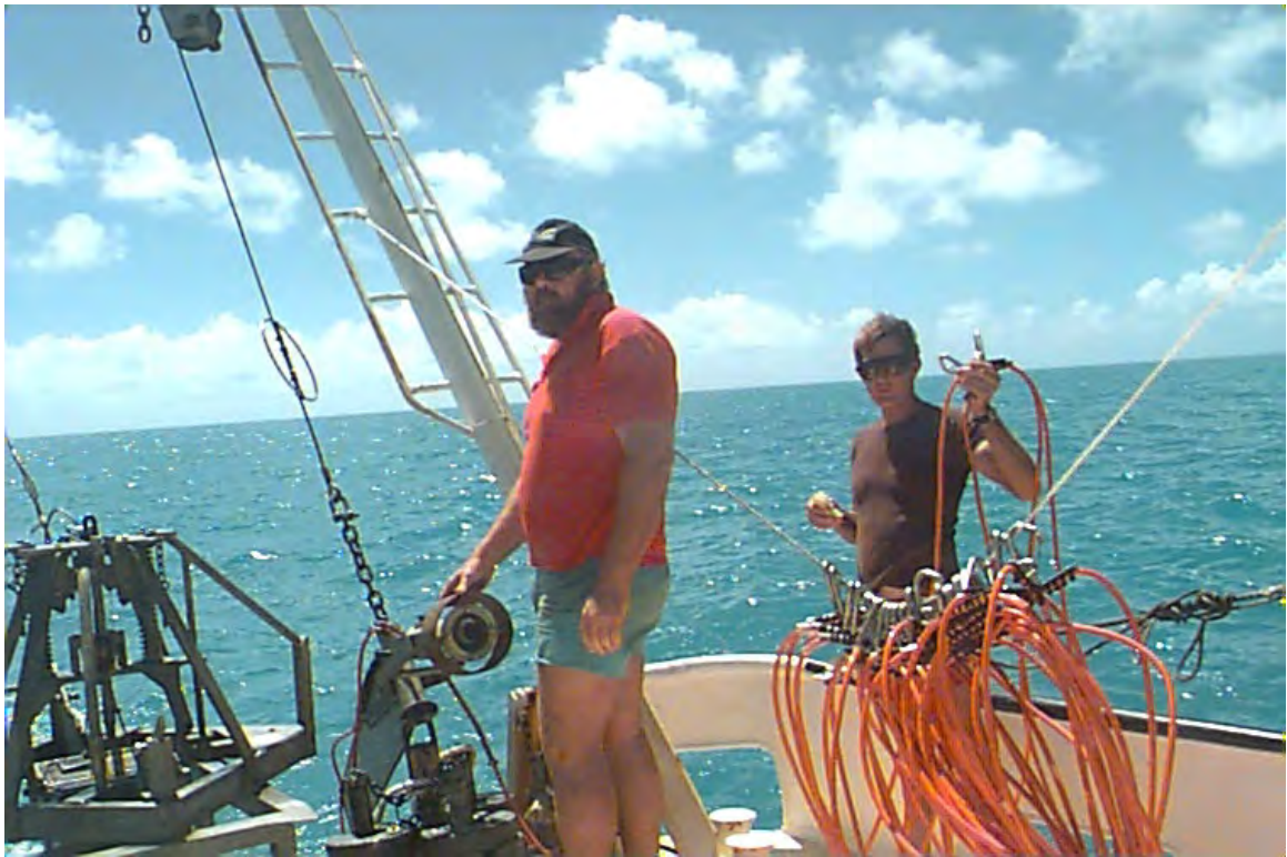
Figure 5–2. Image showing the simple video drop-camera, in water proof housing, suspended from a wire above a heavy weight and a fin to keep the camera facing in the direction of travel. Also shown are the 0.1m 2 Smith-McIntyre sediment grab and video cable to the surface.
