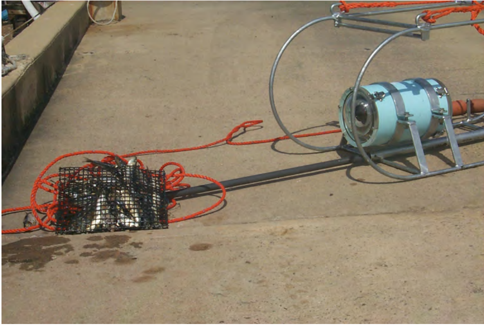
Figure 8–7. Baited Remote Underwater Video Station (BRUVS) with prototype bait arm without measuring grids.
