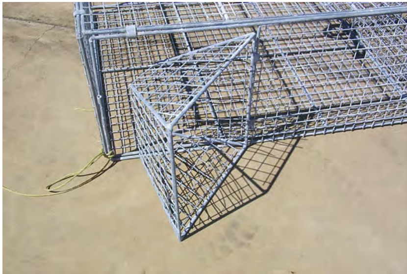
Figure 8-4. Insertion of trap funnel for assembly, bait replacement and catch removal.
