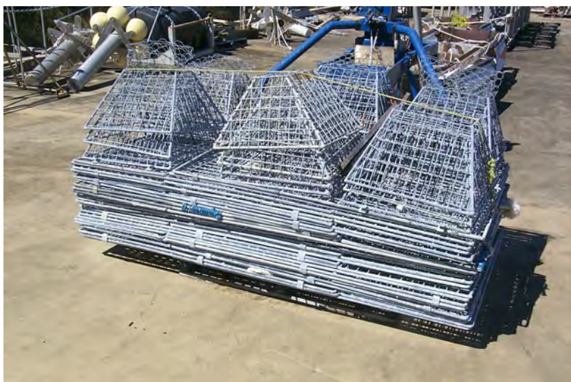
Figure 8-6. Fleet of 10 collapsed traps stacked on shipping pallet.
