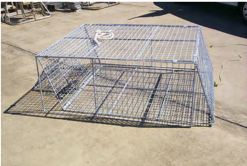
Figure 8–3. Trap assembly pulling top panel along its long axis, and sides fall downward.
