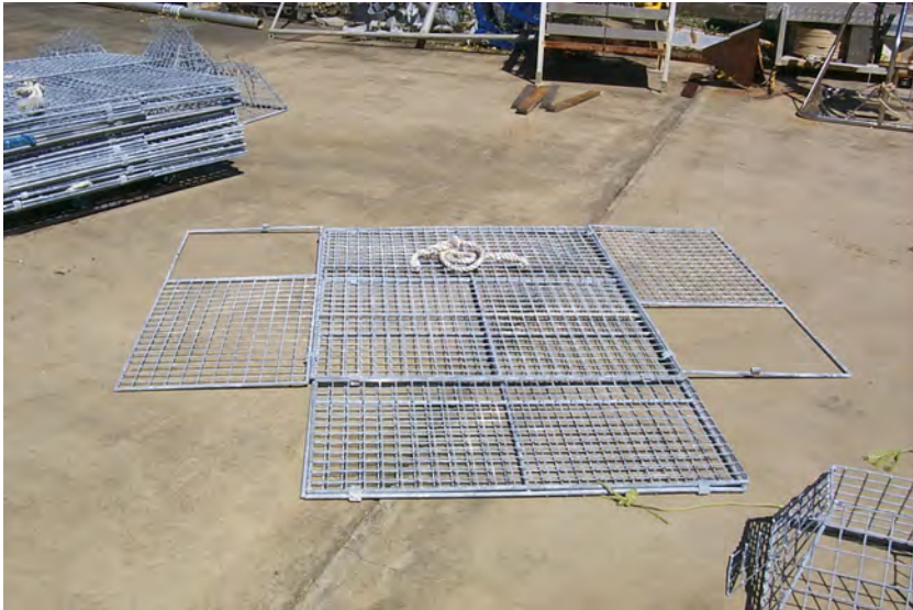
Figure 8–2. (a) Collapsed trap, and (b) with side panels open to start assembly.
